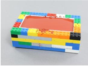
After 3 hours curing time, remove the newplast and master. Make sure all the clay is removed. You can use water to remove the last remnants. Once the silicone is clean and dry, replace the master, cover the surface with a thin layer of talc.
