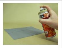
You need to let the paint fall onto the surface rather than spraying it directly onto the surface as with the base coat, this is what creates the speckled effect. If you are using a spray extraction system turn it off so as not to interfere with this process.
