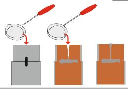
With your gauntlets still on, carefully pour the metal into the channel until it reaches the top of the mould.
