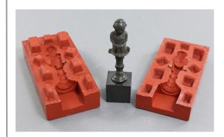
To reproduce a simple figure using silicone rubber.
