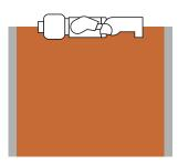
Fill the larger PVC pipe with form sand and press down with your hand.
