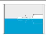
Build a container large enough for your master. Now build a box from 1mm styrene that fits snugly into the container.
