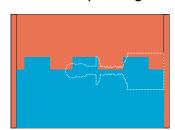
Pour enough silicone to fill the mould a mixing cup. Mix 2-4% (40 drops  $=1g=1cm^3$ ) of catalyst with the resin and mix throughly. When mixed, pour the silicone into the mould and leave to set.
