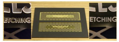
Left & top is a traditional etching on 0.90mm brass whilst the right & bottom is an etching using the new Controlled Etching Technique.
