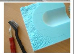
The rough rock texture around the outside of the bowl was created by slashing with the back of the scalpel and also breaking down using a wire brush.
