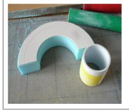
Composite forms in styrofoam (or any rigid material for that matter) are best achieved by deconstructing the intended form into parts or layers to be worked on separately.
