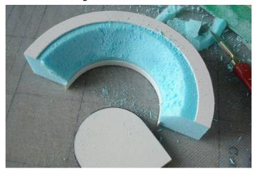
The second part of creating this half-ring shape involves fixing similar 'stops' to the top and base of the blocked shape as shown.
