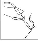
Make sure that the joint surfaces are clean, then add flux and then solder using the iron so each joint surface has a layer of solder.
