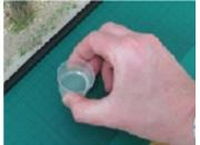
Carefully mix the resin and hardener together making sure you do not introduce bubbles when syringing it into the mixing pot or when stirring the resin and hardener together. When mixed tap the pot to release any small bubbles.
