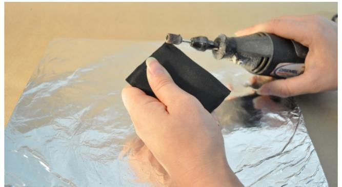
Worbla can be sanded using sandpaper, sanding blocks or a rotary tool.
