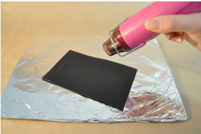
In order to shape and form Worbla you need to heat it. The most common and easiest way to do this is with a heat tool/heat gun.
