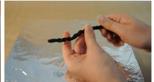
The 'scrap' and left over pieces of Worbla should be kept as these can be heated and then sculpted into shapes in a way similar to working with modelling clay. Larger scraps can also be heated and formed back into a larger sheet by using a rolling pin or iron.
