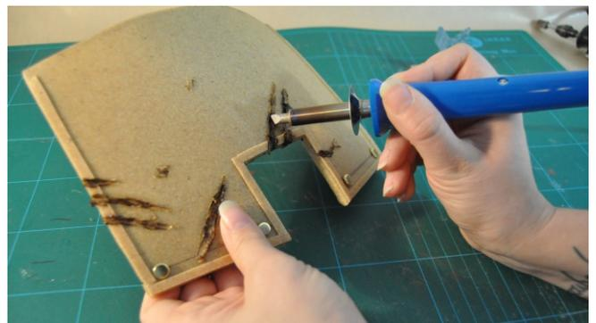
Engraved details (and 'damage') can be achieved by using a rotary or pyrography tool. Adding damage to prop weapons and armour can add realism and 'history' to your project.
